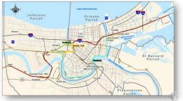
Middle Belt improvements included creating a new route between East Bridge Junction (EBJ) and East City Junction (ECJ) by linking existing, but lightly used rail lines through Jefferson and Orleans Parishes.
