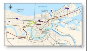
Back Belt improvements included grade separating numerous highway-railroad crossings to improve highway traffic flow and provide additional rail capacity.
